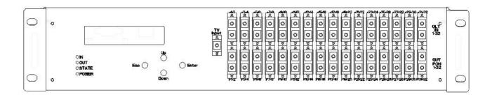
Outline the menu of High Power Optical Amplifier. For the description of all instructions, please refer to the panel shown below. Through the buttons on the right side of the LCD screen, you can scroll through all the menus of the large light.
